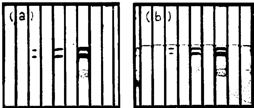
Fig. 2. In PMD, the solvent can be removed by heat alone (a), mainly by gas flush (b), or solely by gas flush. IR radiation (at 5.1 \mu\text{m} wavelength) carries only about 0.05 as much energy per photon as UV at 254-nm wavelength, and so causes little photo-decomposition, but can cause thermal decomposition, in which case solvent is removed mainly or solely by gas. The thermally caused ghost spots shown in (a) are absent in (b) 17 . See also ref. 19. Samples: estrone, estradiol, and estriol, 0.5 mg/ml each, in methanol. Spotted volumes: 1, 5 and 10 \mu\text{l} . Plates: Quantum Q5DF.
